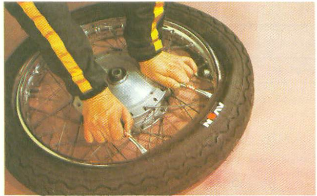
Use two levers to work bead over the edge of rim
