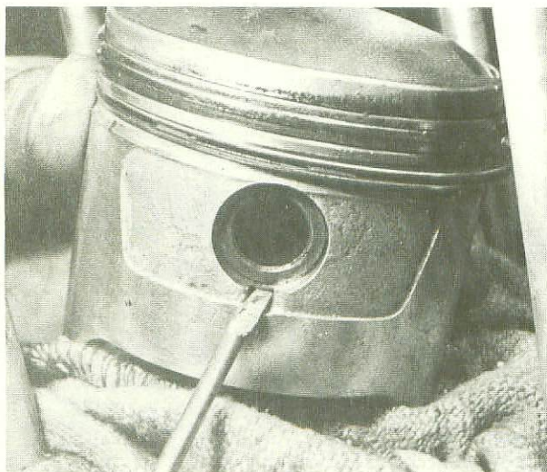
8.1 Prise in groove to release circlip
