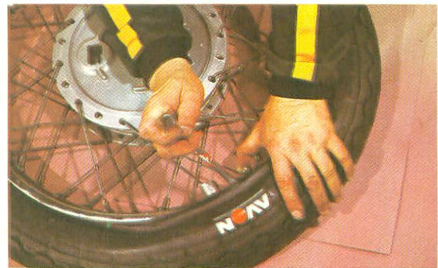
Push valve and tube up into tyre when fitting final section, to avoid trapping
