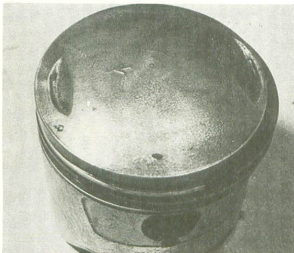
32.2 Arrow points towards front of engine
