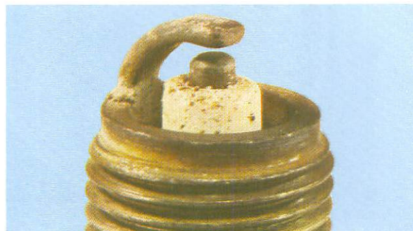
A blistered white insulator or melted electrode indicates over-advanced ignition timing or a malfunctioning cooling system. If correction does not prove effective, try a colder grade plug
