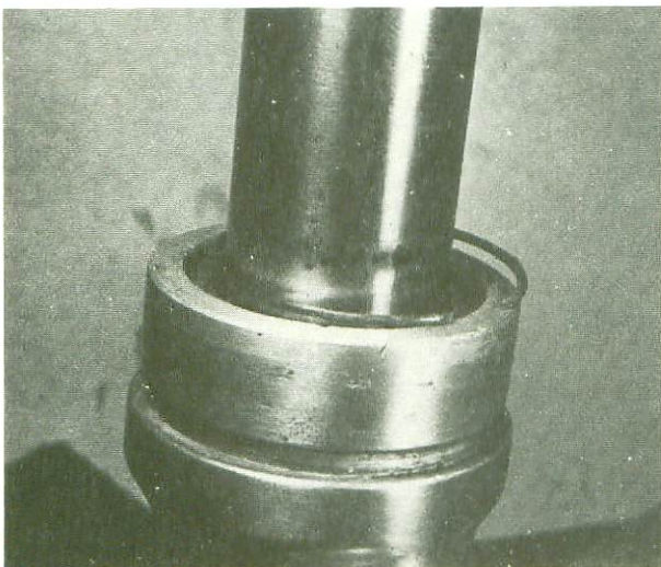
3.7A Take out circlip
