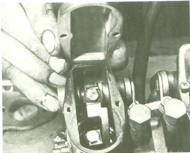
5.6 Slide should be easy in bore
